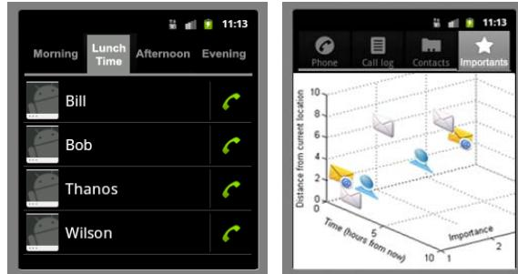
Figure 6a (left) and 6b (right). Retrieval UIs using 2D (left) and 3D (right) projections of item (contacts, e-mails, photos etc.) importance combined with retained, unprojected dimensions (time, distance from current location).
