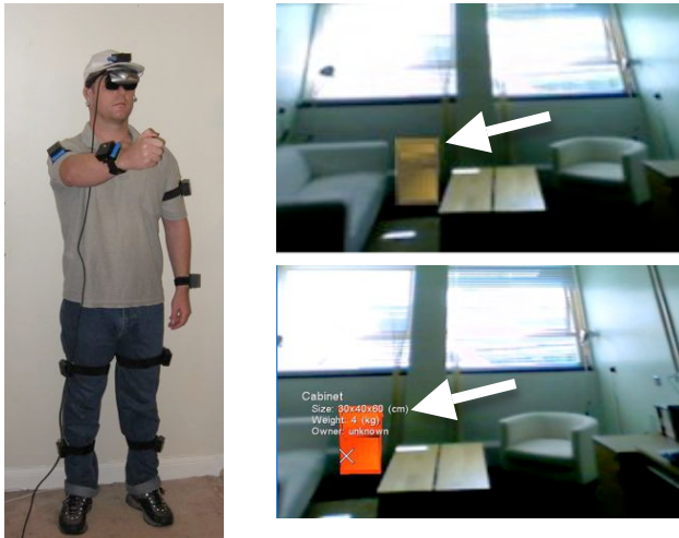
Figure 4. The user points an arm-controlled cursor (visualized to the user as an X) at the virtual object (marked by the white arrow), which is then highlighted. Metadata for that object is subsequently displayed.
