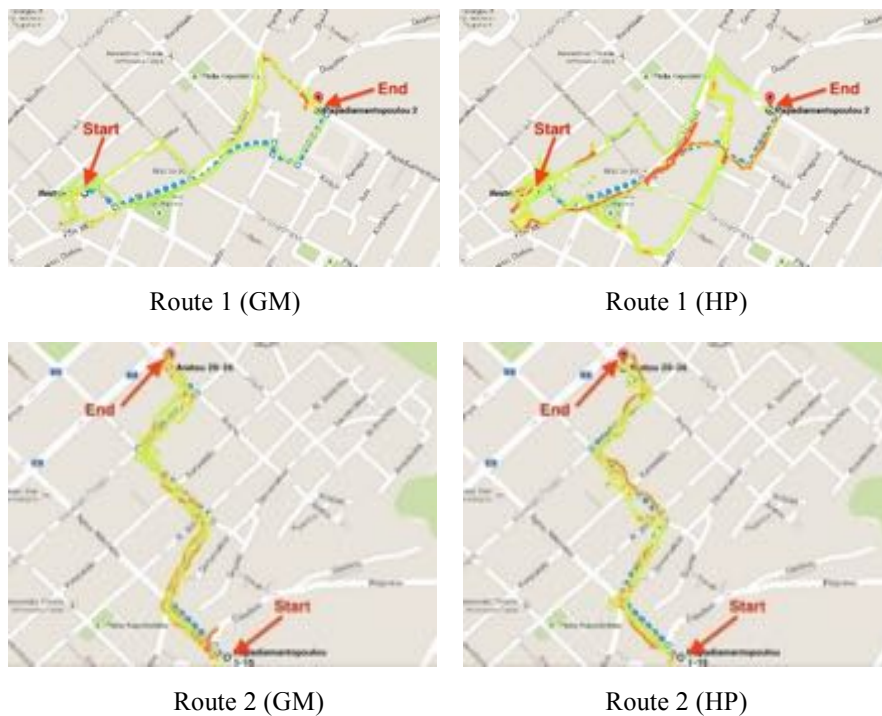
Fig. 2. Participant Routes and heatmapped GPS traces. The red segments show where participant speed was less than 1 km/h
