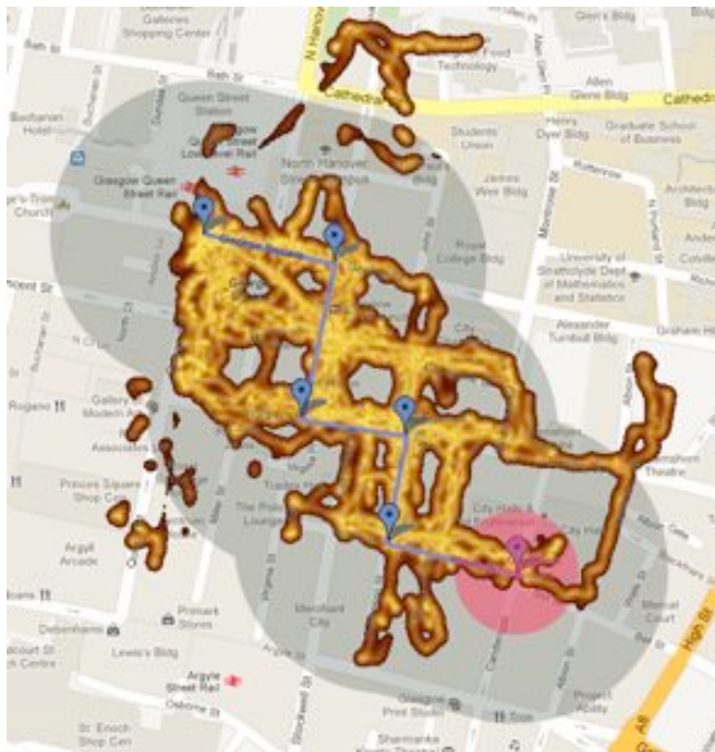
Figure 11. Heat map of all participants' GPS traces superimposed on the audio scent zone of coverage (shaded grey area), clearly showing the islands of GPS data (errors)
