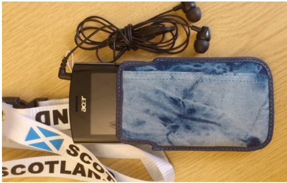
Figure 8. The equipment worn by participants. It consists of an Acer Liquid Metal Android device with integrated GPS & magnetic compass, a soft fabric case, neck strap and in-ear Sony headphones.
