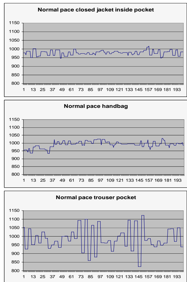
Figure 2: Examples of data output from various device positions (Y axis shows acceleration in milliG, X axis is the reading id)
