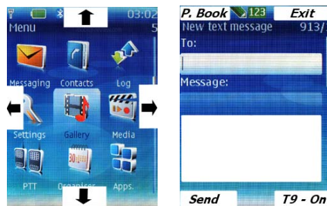
Fig. 1. A mock-up of cursor control is shown on the left. The mock-up on the right shows four commands at the corners of the screen. A user might “blink to click” any of the commands, or “blink to move” to the text input fields. The command areas might be context-sensitive, with different commands displayed, according to the user's current control focus.
