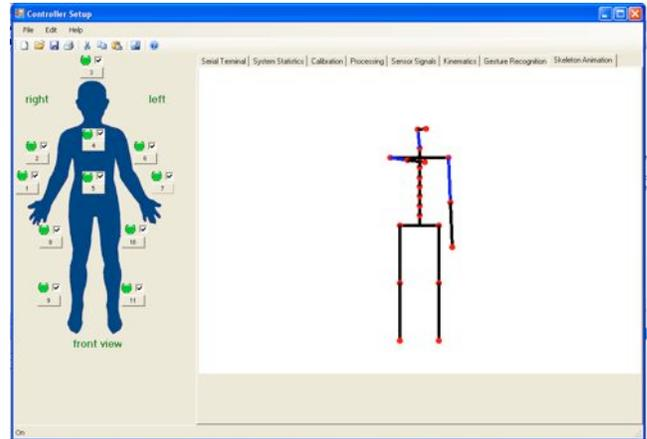
**Figure 2. The motion capture interface (PC). A user can indicate which sensor packs are being worn by checking the relevant boxes on the human outline shape. The green status dots turn red when the sensor pack is not transmitting. The skeleton model on the right is constructed in real-time.**
