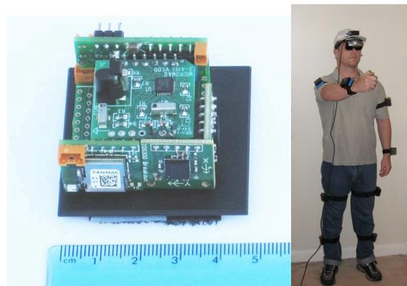
**Figure 1. Our custom-designed sensor pack containing 3-axis accelerometer, gyro, magnetometer and 802.15.4 comms (left). On the right, a user demonstrating the small size and wearability of the packs, Velcro-strapped on his body. The cable attaches his VR headset to the host PC.**
